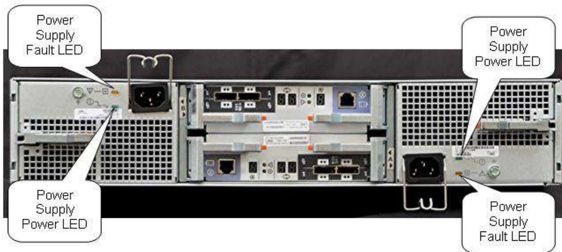
Figure 8. Back of the 25-drive DAE housing 2.5" drives
