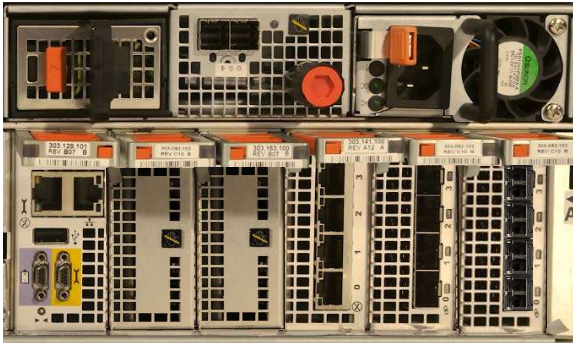
Figure 26. A close-up of the back of the DPE-based storage processor
